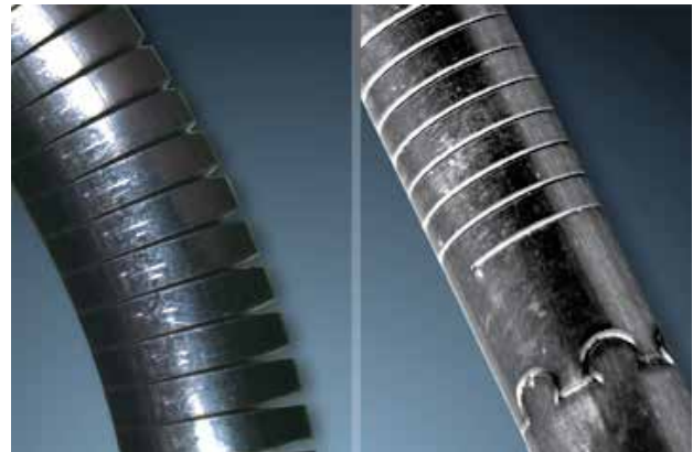
Laser cut flex patterns with other attachment forms for laser welded assemblies.
