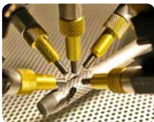
Automated microblasting treatment
